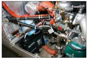
It is necessary to abide by the polarity of the battery and the battery charger. It may destroy the battery if the polarity is changed. It is recommended to disconnect the battery before charging!!!
