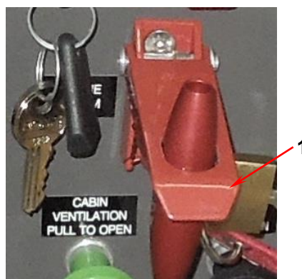
Fig. 3.8.4-1 Emergency system actuator protector
