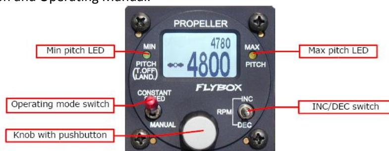
Fig. 7.9-2 Propeller regulator
