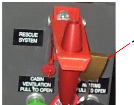
Fig. 4.5.1-1 Emergency system actuator lock
